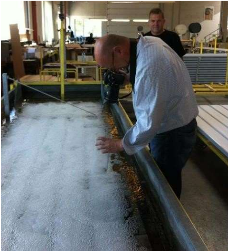
Figure 6 Each AEROSTRIP® is tested for permeability, hole density and pressure loss prior to dispatch
